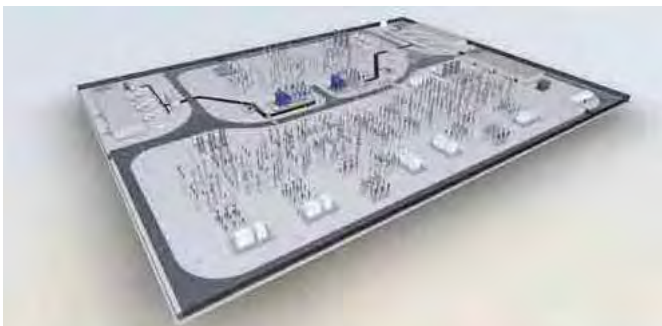
Indicative view of an AIS Substation
