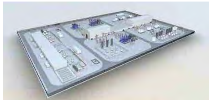
Indicative view of a GIS Substation
